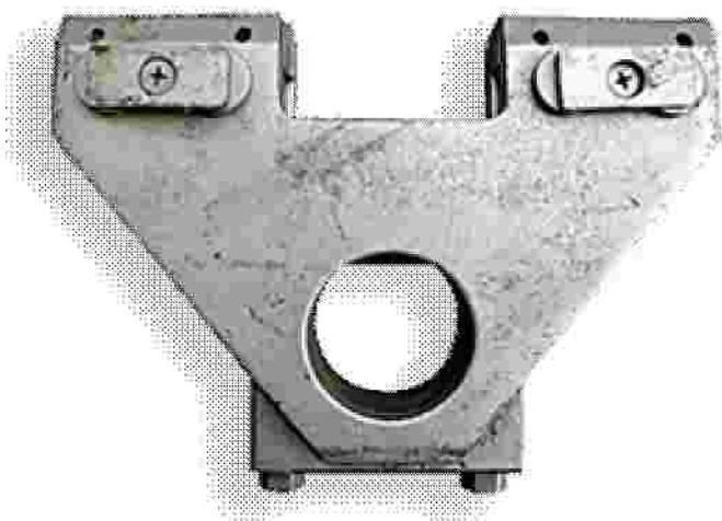
This is a commercially available "Pinch Weld Clamp" which clamps to a rocker panel or other pinch weld and can then be bolted to the Chassis Jig or used to pull part of the vehicle into alignment.
